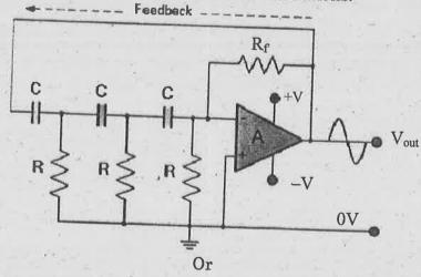
(b) Find the loop transmission L(s) and the characteristic equation for the positive-feedback circuit shown below. Sketch a root-locus diagram for varying K, and find the value of K that results in a maximally flat response and the value of K that makes the circuit oscillate. Assume that the amplifier has frequency-independent gain, infinite input impedance, and zero output impedance.
